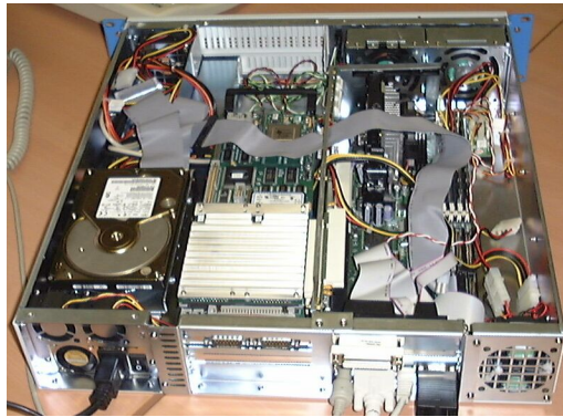
Figure 6.12: Small cabinet with improved air flow due to multiple fans with M67/AD16 board equipped with heat spreader
