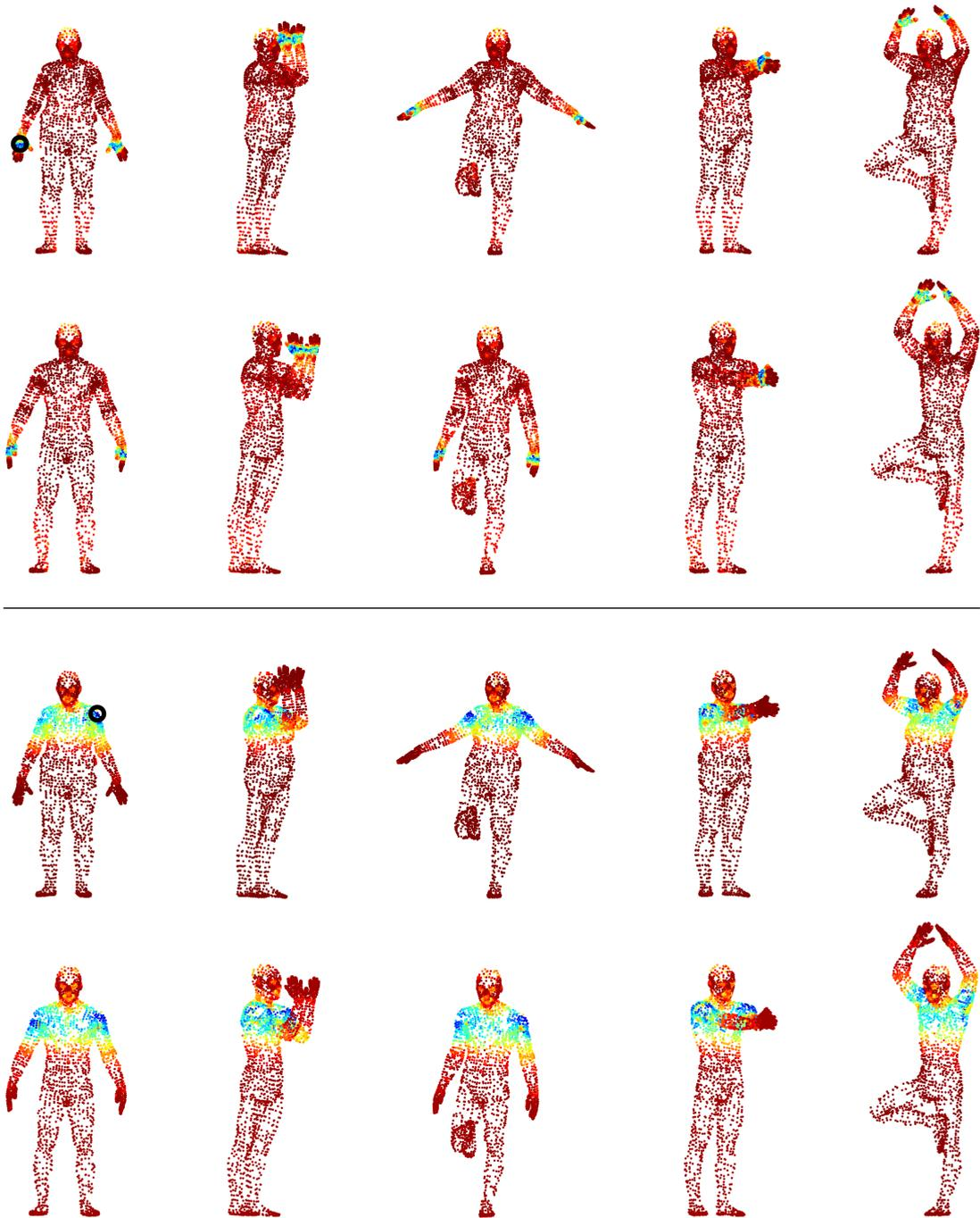
**Fig. 4.3:** Visualisation of distances in the descriptor space between all points on a selection of shapes from the FAUST test set and a single point  $\bullet$  on a reference shape (upper left). Cold colors correspond to small distances. Distances are saturated at the median.
