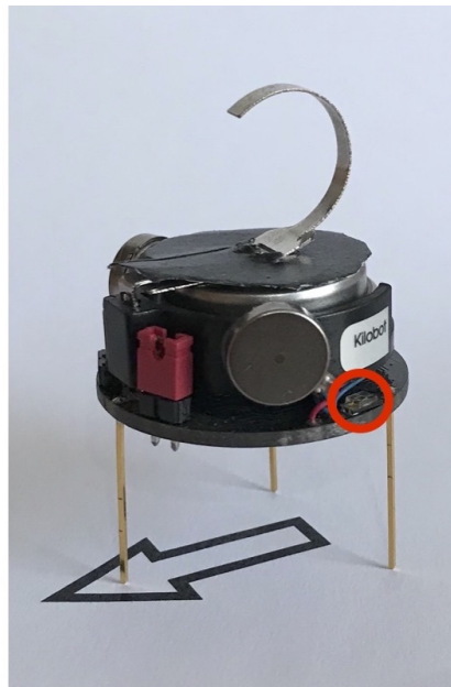
Fig. 3.1 A Kilobot is shown with its heading direction indicated by an arrow and its light sensor by a red circle.
