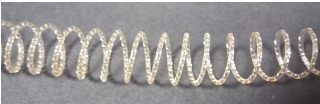
Fig. 5.12 Large diameter coil muscle with 18 mm diameter and 20 cm length
