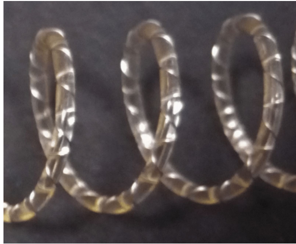
Fig. 5.15 Closeup heating wire
