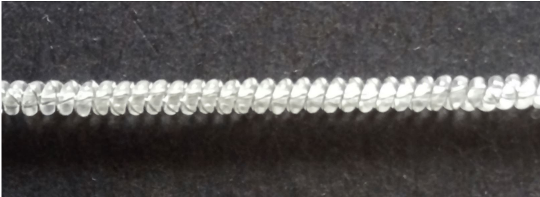
Fig. 5.11 Coiled muscle with 1.6 mm diameter and 20 cm length
