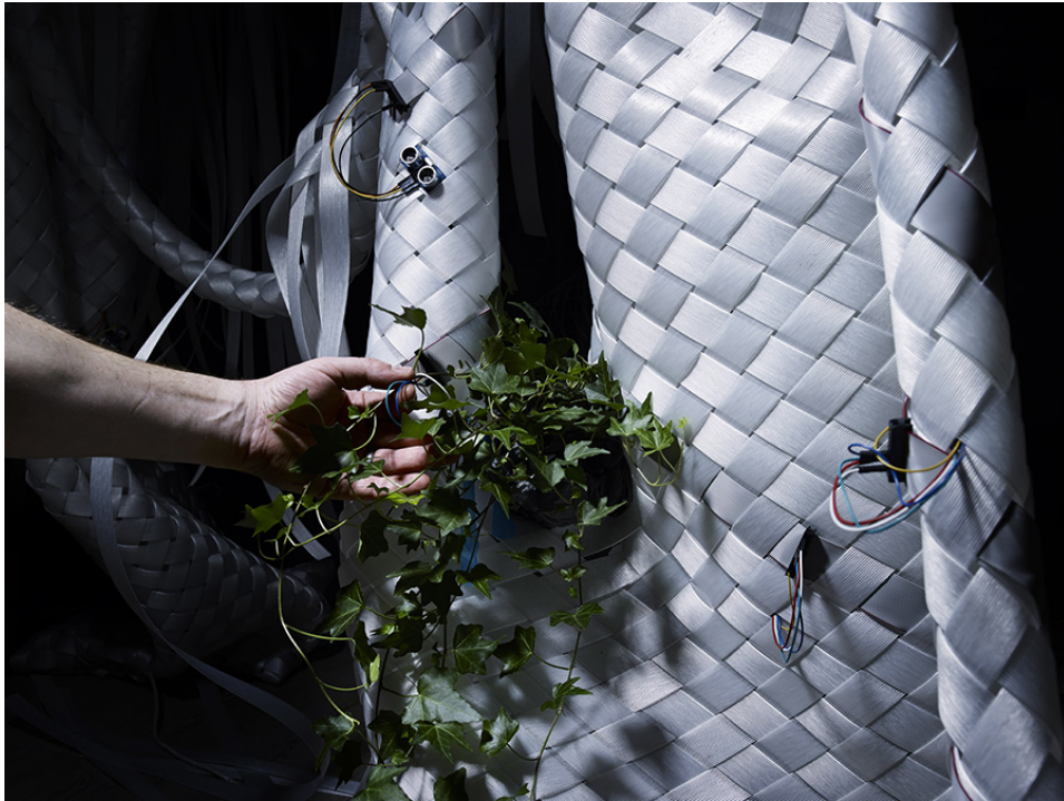
Fig. 2.7 A braided structure with a prototype of electronics-embedded filaments.
