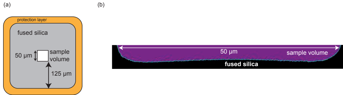
Figure 3.3: (a) Schematic cross-section of the fused silica capillary with polyimide protection layer (orange), roughly to scale. (b) Photo of the inner wall of the capillary made with a digital microscope (VHX-5000, Keyence).
