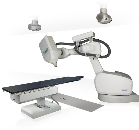
Figure 1.3: The CyberKnife® radiosurgery system showing the LINAC mounted on the industrial robot, the robotic couch, and the stereoscopic X-ray sources and floor detector. Image courtesy of Accuray Incorporated - © [2015] Accuray Incorporated. All Rights Reserved.
