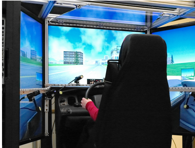
Figure 6.13: View of the state-of-the-art FAAC driving simulator. The system emulates the interior of a car, in which the windshield, covering a 225 degrees horizontal field-of-view, is created using five LCD panels. The simulator is integrated with a six-camera Smart Eye PRO eye tracking system.
