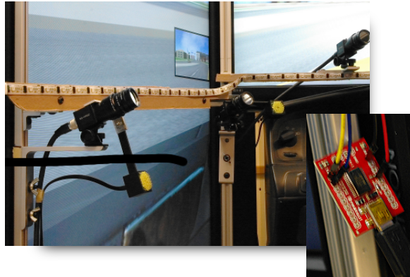
Figure 6.15: LED strip mounted on aluminium profiles across the bottom edge of the simulated windshield. Thumb image: the breakout board used to connect the LED array to the controller unit.
