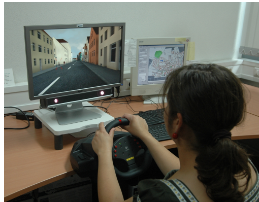
Figure 6.2: Still shot from a simulator recording. The remote eye tracker that was integrated to the driving simulator is visible below the screen. The subjects controlled the simulation using a pedal/steering wheel system. The DS server, displaying the map of the simulated environment, is visible to the right of the image.
