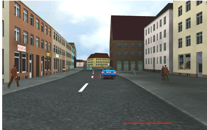
Figure 6.9: Stillshot from the second experiment. The GCC highlights the direction from which the high-risk pedestrian is walking. As before, the cues are only activated if the driver is not looking in the direction of the critical event, and they disappear when the driver fixates the pedestrian in question.
