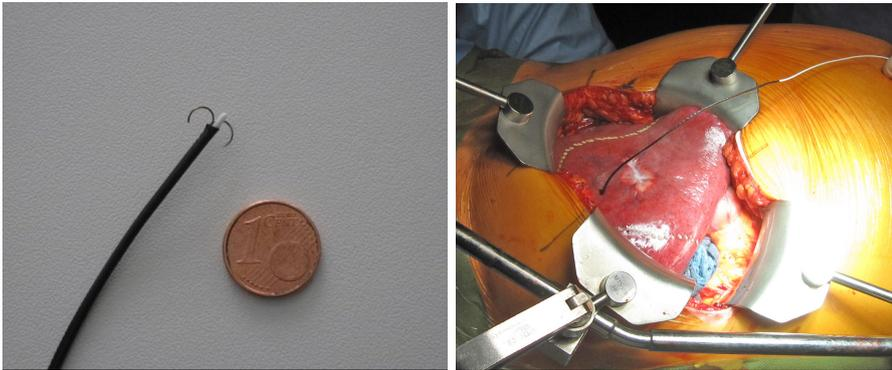
**Figure 2.16** The size of a small anchor sensor coil compared to a one cent coin (left) and inserted into the liver during a resection (right).
