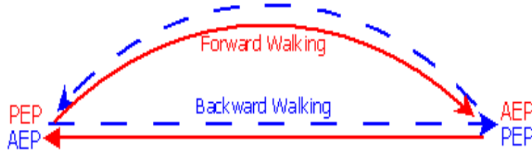
FIGURE 6.4.1. The direction of leg trajectory during the swing and the stance phase in case of forward and backward walking. The red curve represents the leg trajectory in forward direction. The blue curve represents the leg trajectory in backward direction.
