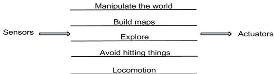
FIGURE 3.3.1. Reactive and Behavior-Based Architecture [24].
